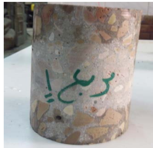
Fig. 5. Core specimen cut from square column
